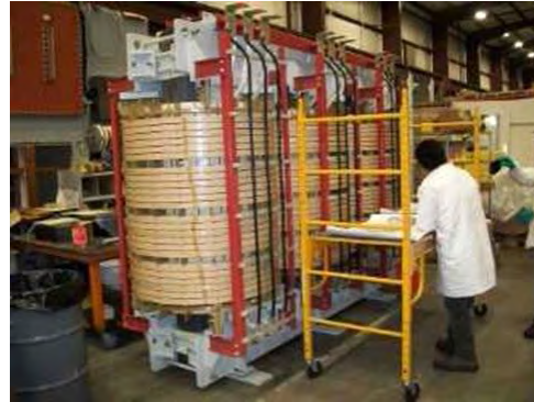
Figure 1 DTI and Neeltran 4.3 MW, 7 MVA, 24 pulse transformer rectifiers that DTI installed at the integrated system at the Army Corps of Engineers facility in Romeoville, Illinois
