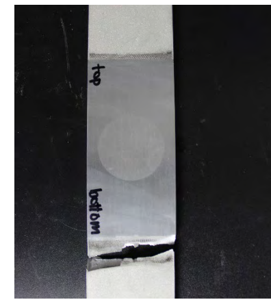
Grip Failure R= 0.1 N= 38,524 cycles
